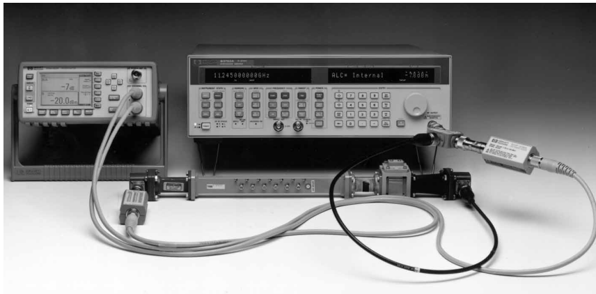
Figure 5-7. HP E4419A dual-channel power meter measures insertion loss of a 11.245 GHz waveguide bandpass filter, using its power ratio mode, plus a sweeper and power splitter. HP's 90-dB dynamic-range sensors are ideal for such high-attenuation measurements.
