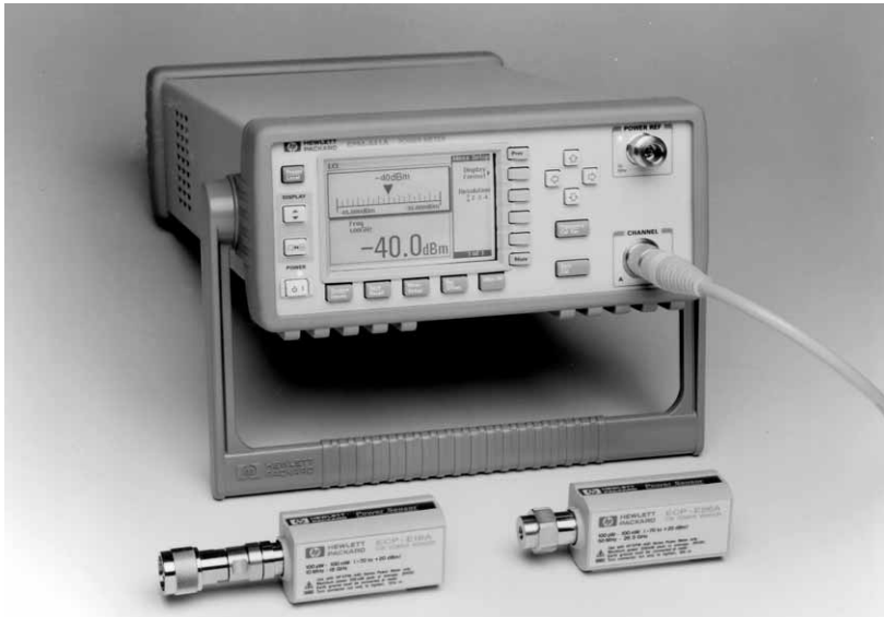
Figure 4-11. HP E4418A features many user-conveniences and a 90 dB dynamic measurement range.
